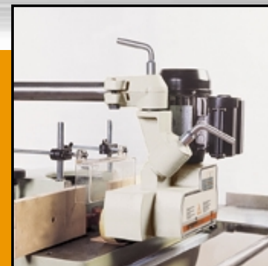
▲ Power feeder positioned on a spindle moulder
