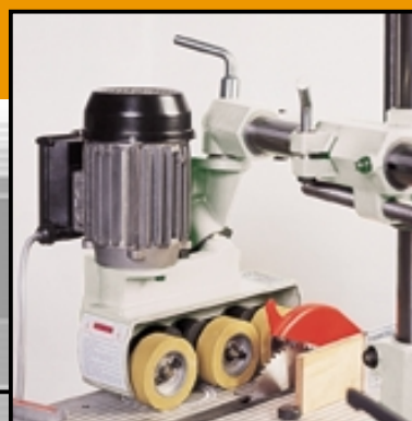
▲ Power feeder positioned on a circular saw
